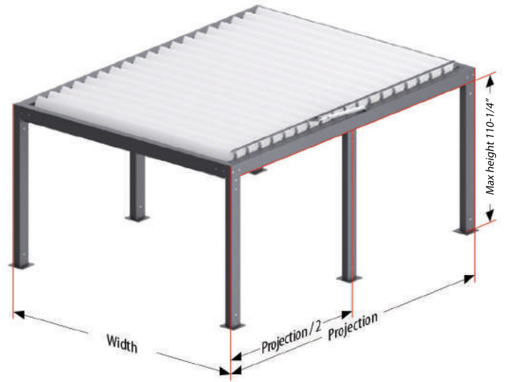
Version II for pergola with over 204-1/4" projection includes a middle pole supporting the construction
